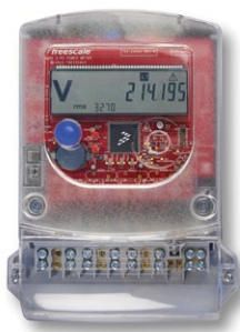
Electronic Tamper Detection Smart Meter Reference Design Using MMA8491Q Xtrinsic Tilt Threshold Sensor
