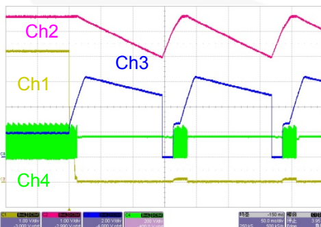
Figure 33. 120V AC / 60Hz at Max. Load (Ch 1: V O , Ch 2: V CC , Ch 3: V FB , Ch 4:V DS )
