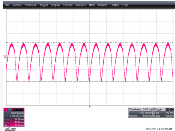
Figure 27. V_{O\_RIPPLE} = 64.8\text{mV} , Maximum Output Ripple at 265\text{V}_{AC} , CH2: V_O (20mV/div), Time: 1ms/div
