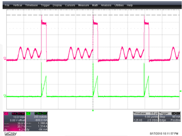
Figure 18. V_{DIODE,MAX} at Normal = 35.7V, 5V Output Diode with 265V AC & Full-Load Condition, CH2: V_{DIODE} (10V/div), CH4: I_{DS} (200mA/div), Time: 5µs/div
