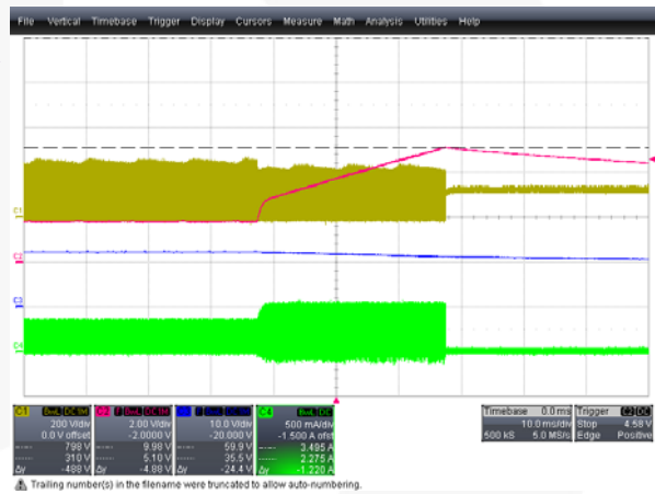
Figure 28. OLP Triggered: V_{FB} = 5.10\text{V} , Output Short with 90\text{V}_{AC} and Full-Load, CH1: V_{DS} (200V/div), CH2: V_{FB} (2V/div), CH3: V_{CC} (10V/div), CH4: I_{DS} (500mA/div), Time: 100ms/div and 10ms/div
