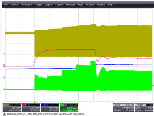
Figure 10. Soft-Start, 265V AC and Full-Load Condition, (CH1: V_{DS} (200V/div), CH2: V_{FB} (2V/div), CH3: V_{CC} (10V/div), CH4: I_{DS} (200mA/div), Time: 2ms/div
