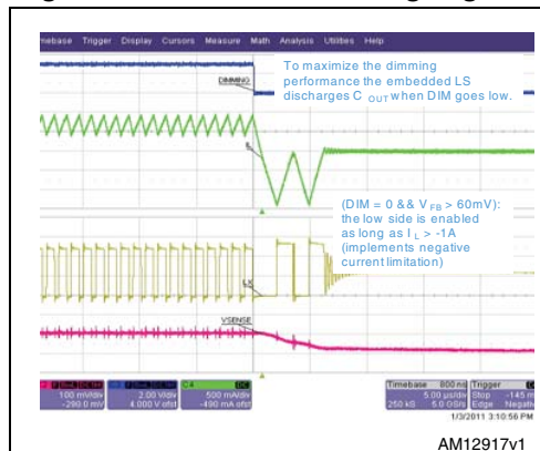
Figure 28. LED current falling edge
