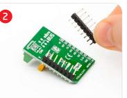
Turn the board upside down, so that bottom side is facing you upwards. Place shorter parts of the header pins in the both soldering pad locations.
