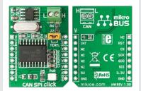
CAN SPI click 5V is an accessory board in **mikroBus**<sup>Im</sup> form factor. It is the best solution for adding CAN connectivity to your microcontroller with SPI interface. Board features **MCP2551** CAN transciever circuit which provides CAN serial communication physical layer in accordance with the ISO 11898 standard. It is designed for operation in especially-harsh environments, providing reliable solution. Board is designed to use 5V power supply only.
