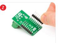
Turn the board upside down, so that bottom side is facing you upwards. Place shorter parts of the header pins in the both soldering pad locations. Turn the board upward again. Make sure
