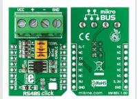
RS485 Click 3.3V is an accessory board in **mikroBus**<sup>III</sup> form factor. The on-board **SN65HVD12** differential line transceiver is suitable for high speed bidirectional data communication on multipoint bus transmission lines. It is designed for balanced data transmission and complies with EIA RS-485 standard. This transceiver features a differential line driver and differential line receiver. Board is set to use 3.3V power supply only.
