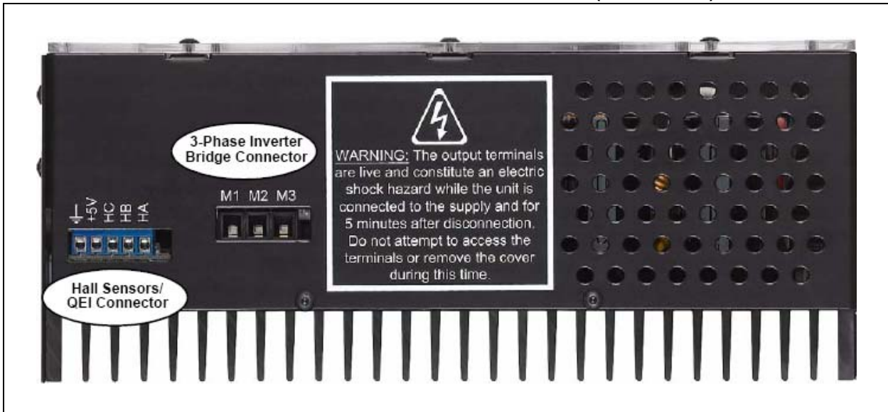
FIGURE 2-4: dsPICDEM™ MCHV-2 DEVELOPMENT BOARD (RIGHT SIDE)
