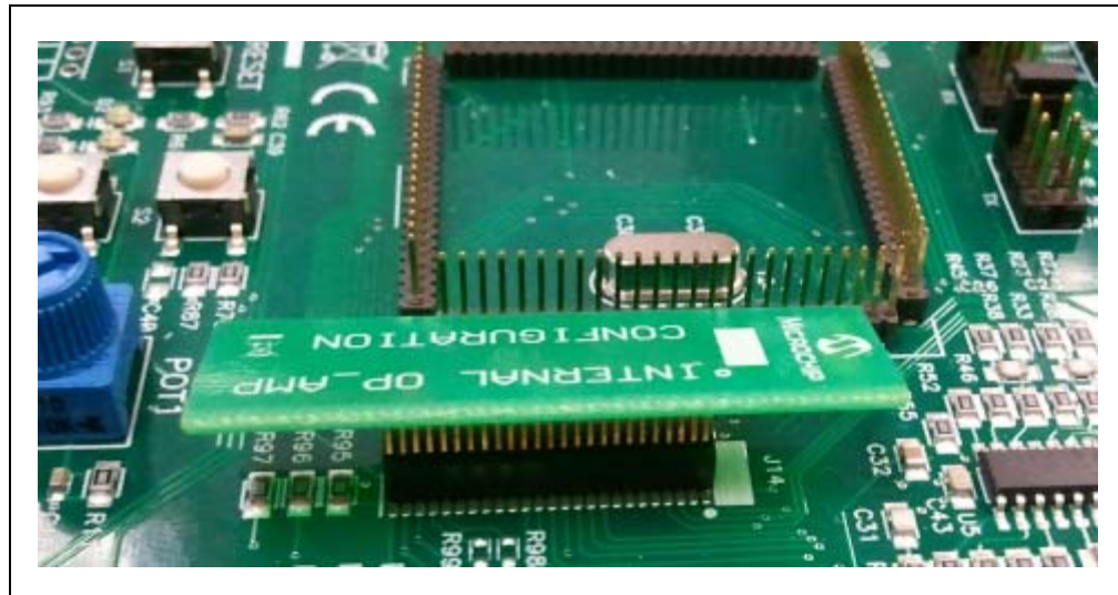
FIGURE 3-1: MATRIX BOARD ORIENTATION
