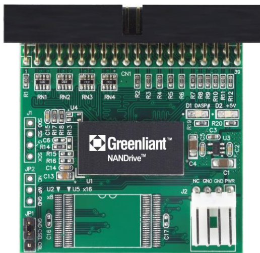
Figure 1: NANDrive Evaluation Board, 40-pin Connector
