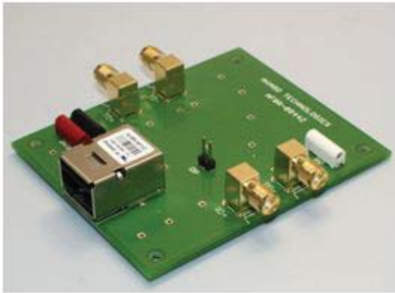
Figure 1. Evaluation board for the AFBR-5972Z transceiver module
