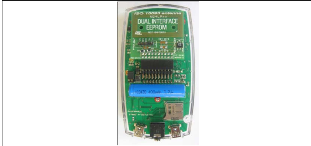
Figure 50. Connecting your reference antenna to your STM32-PRIMER2
