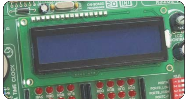
Figure 29 2x16 LCD in 4-bit mode
