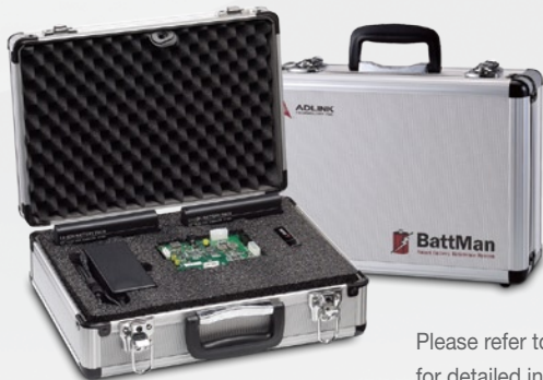
BattMan Smart Battery Management Reference System
