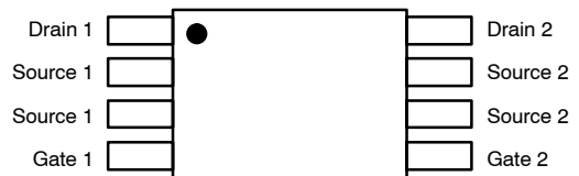
Figure 3. Pinouts for Dual-Die TSSOP
