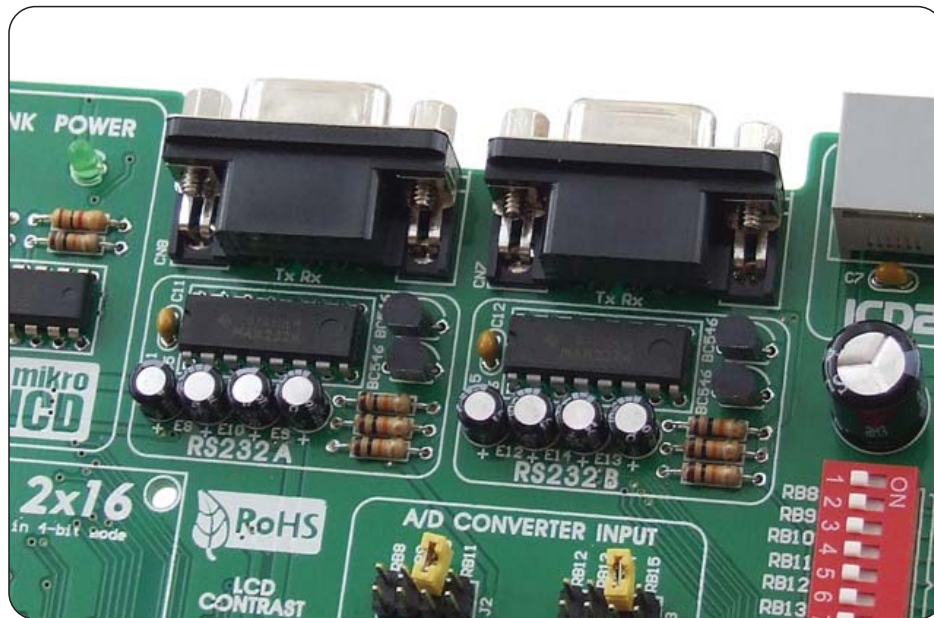
Figure 10 RS-232 communication ports
