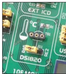
Figure 10-2: J11 in the left-hand position (1-wire communication through the RA5 pin)
