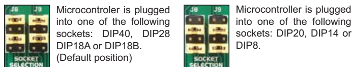
Figure 3-5: The position of jumpers J8 and J9
