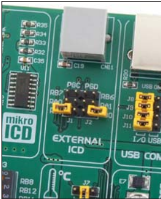
Figure 5-1: ICD connector (default position)
