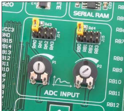
Figure 7-1: A/D converter (jumpers in default position)
