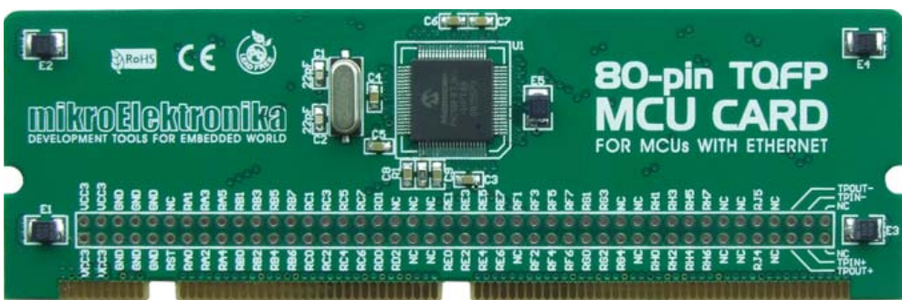
Figure 2-3: MCU card with 80-pin microcontroller in TQFP package soldered on it
