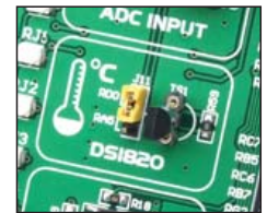
Figure 14-4: DS1820 is connected to the microcontroller via the RD0 pin
