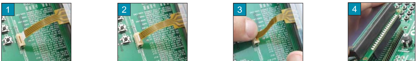
Figure 20-3: Placing touch panel
