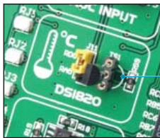
Figure 14-2: DS 1820 is plugged into the connector
