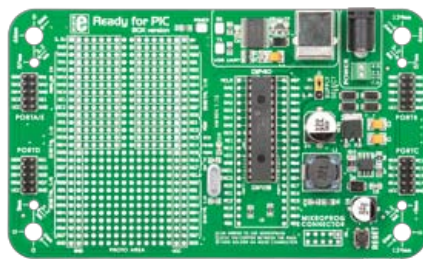
02 Ready for PIC® board with male pin headers
