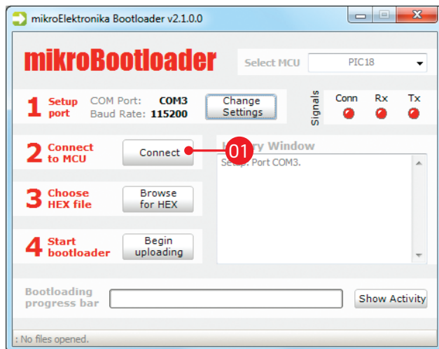
Figure 2-4: Connecting with mikroBootloader
