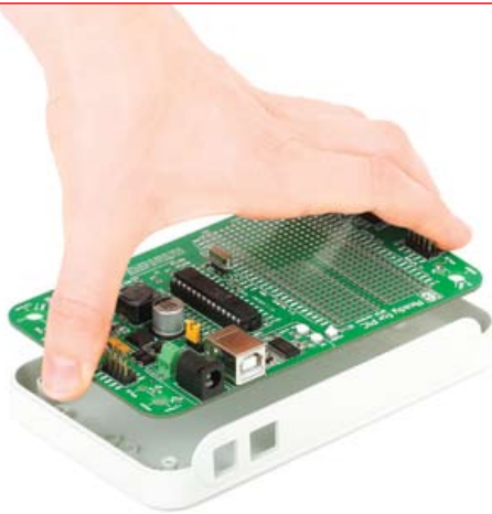
Figure 8-1: Place the board into the bottom part of the casing. Make sure that connectors are aligned with square openings
