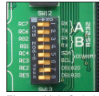
Figure 11-3: Switch 7 on the DIP switch SW12 is in ON position, DS1820 is connected to the PE2 pin
