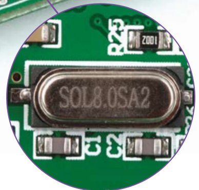
Figure 5-1: External crystal oscillator (X1)
