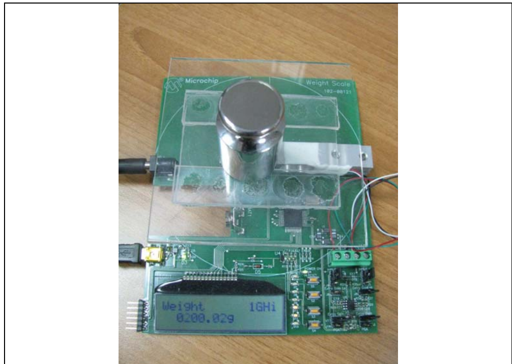
FIGURE 1-1: MCP3421 Weight Scale Demo Board.
