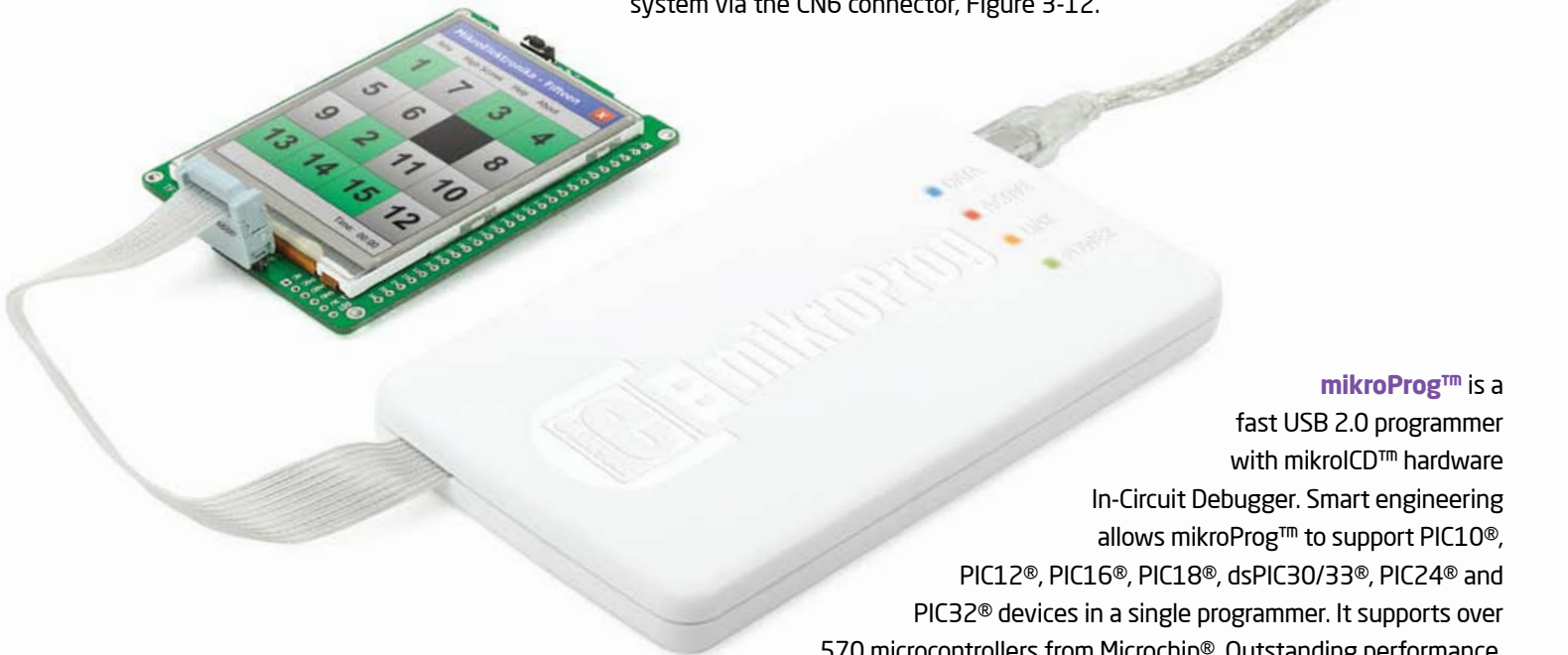
Figure 3-12: Connecting mikroProg™ to mikromedia™
