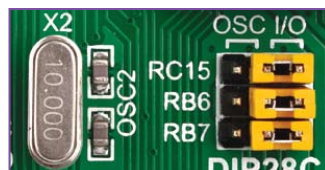
Figure 4-8: RC15, RB6 and RB7 as I/O pins (when using internal oscillator)
