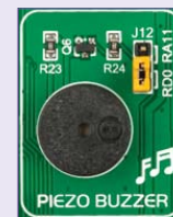
Figure 19-2: Use jumper J12 to connect Piezo buzzer on R20 or RA11 pin
