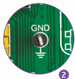
Figure 20-1: 3 oscilloscope GND pins are conveniently positioned so each part of the board can be reached with an oscilloscope probe
