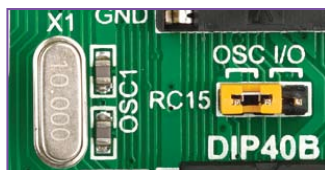
Figure 4-7: RC15 connected to X1 quartz-crystal
