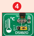
Figure 12-4: DS1820 connected to G2.0 pin
