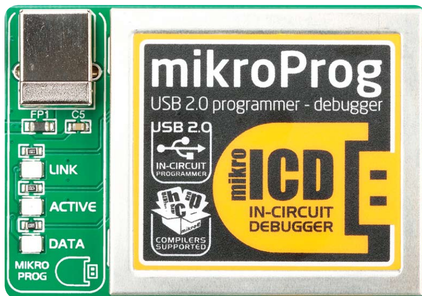
Figure 5-1: mikroProg™ is well protected under metal casing
