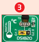
Figure 12-3: DS1820 connected to G1.7 pin
