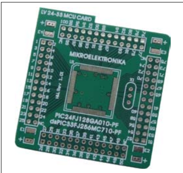
Figure 20: Empty MCU card MCU Card 7
