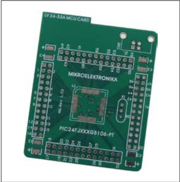
Figure 38: Empty MCU card MCU Card 13
