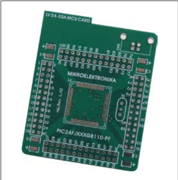
Figure 47: Empty MCU card MCU Card 16
