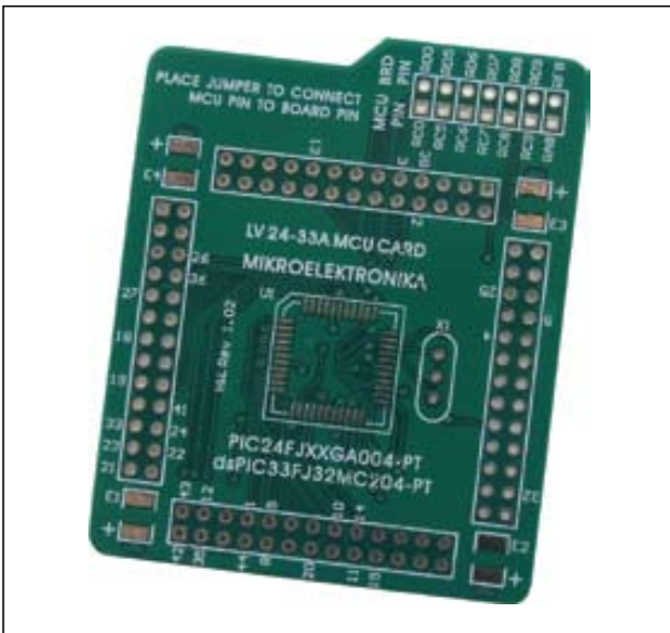
Figure 35: Empty MCU card MCU Card 12
