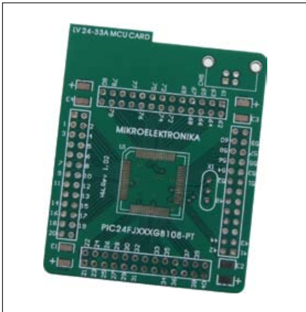
Figure 41: Empty MCU card MCU Card 14
