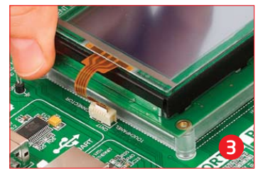
Figure 14-3: Now place GLCD with Touch panel into GLCD socket
