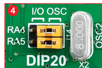
Figure 4-9: RA4 and RA5 connected to X2 quartz-crystal
