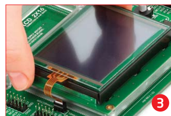
Figure 13-3: Now place GLCD with Touch panel into GLCD socket
