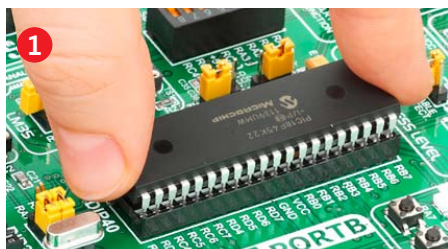
Figure 4-3: Place both ends of microcontroller on the socket so the pins are aligned correctly
