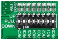
Figure 10-2: Tri-state DIP switch on PORTC
