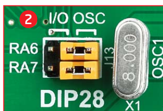
Figure 4-7: RA6 and RA7 connected to X1 quartz-crystal
