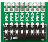
Figure 6-2: Tri-state DIP switch on PORTE
