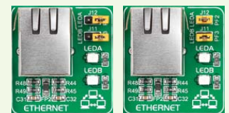
Figure 12-2: Enabling ethernet LEDs (photo on the right)
