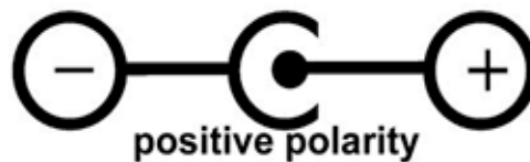
Figure 2-1. Power Supply Barrel Connector (J2) Polarity
