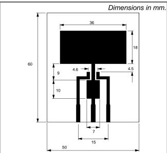
Fig.4. PCB for thermal resistance and power rating. PCB: FR4 epoxy glass (1.6 mm thick), copper laminate (35 μm thick).
