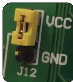
5V while button is pressed
