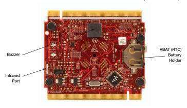
Figure 2: Back side of TWR-K20D50M module.
