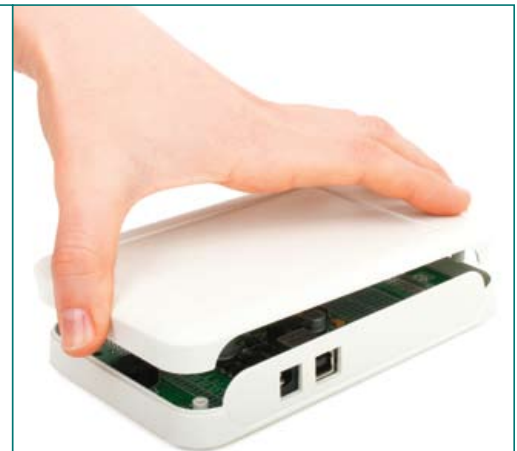
Figure 9-2: Place cover casing plastic and wind screws into outer screw holes for connecting it with bottom plastics
