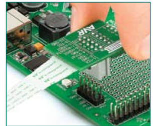
Figure 3-12: connecting JTAG programmer
