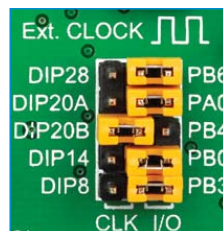
Figure 4-8: Position of the jumpers for DIP20B
