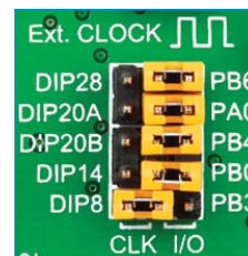
Figure 4-10: Position of the jumpers for DIP8
