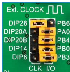
Figure 4-6: Position of the jumpers for DIP28
