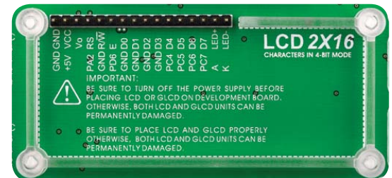
Figure 10-1: On-board LCD 2x16 display connector
