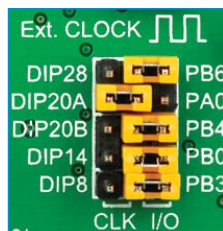
Figure 4-7: Position of the jumpers for DIP20A
