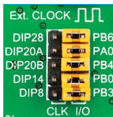
Figure 4-5: Position of the jumpers for DIP40x
