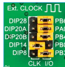
Figure 4-9: Position of the jumpers for DIP14
