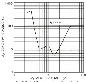
Fig. 5 Typical Zener Impedance Characteristics
