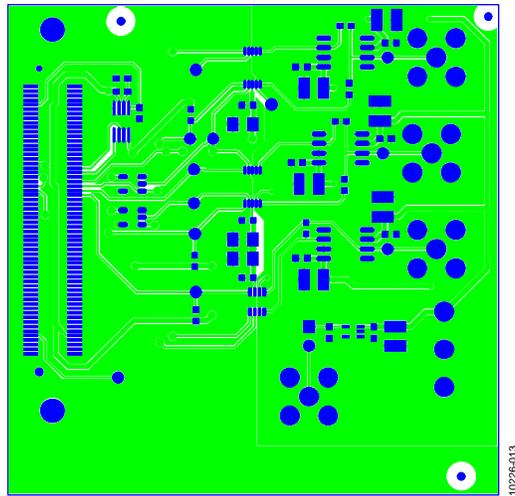
Figure 13. EVAL-AD5443SDZ/EVAL-AD5446SDZ/EVAL-AD5453SDZ Component Side
