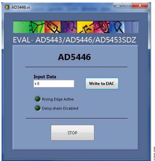
Figure 6. AD5446 Evaluation Software Window
