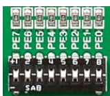
Figure 6-2: Tri-state DIP switch on PORTE
