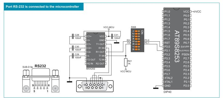
Figure 6-2: RS-232 module schematic
