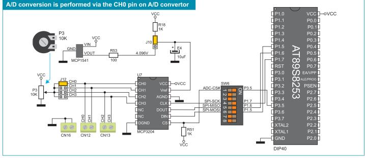
Figure 7-3: Microcontroller and A/D converter test inputs connection schematic
