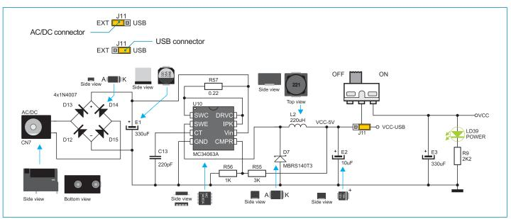
Figure 5-2: Power supply source connection schematic
