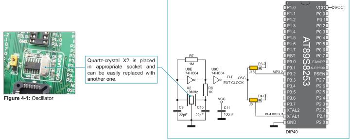
Figure 4-2: Oscillator schematic
