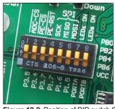
Figure 18-2: Position of DIP switch SW6 when the port expander is enabled
