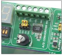
Figure 7-1: ADC (jumper default position)
