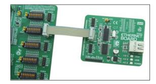
Figure 1-3: Placing additional modules on the board
