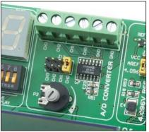
Figure 7-2: Pin CH0 used as A/D conversion input
