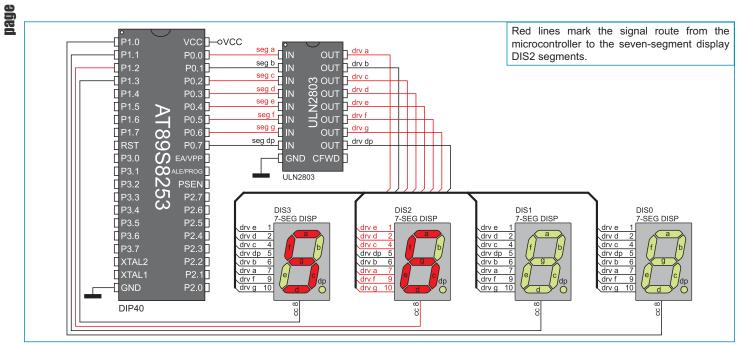
Figure 16-3: Showing a digit on the seven-segment display DIS2
