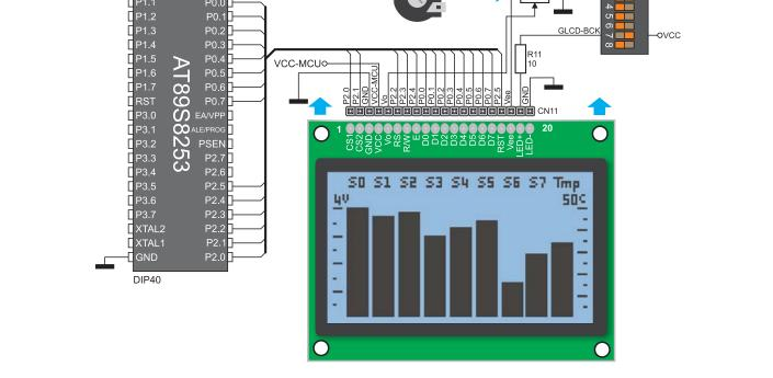
Figure 15-3: GLCD display connection schematic
