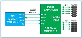
Figure 18-3: SPI communication block diagram
