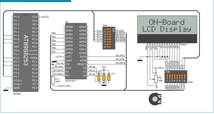
Figure 13-2: On-board LCD display connection schematic
