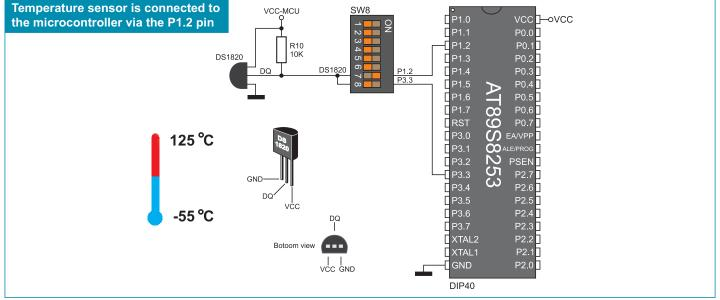
Figure 8-5: DS1820 and microcontroller connection schematic
