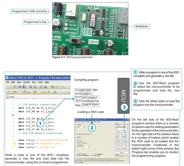
Figure 3-2: The principle of the programmer's operation
