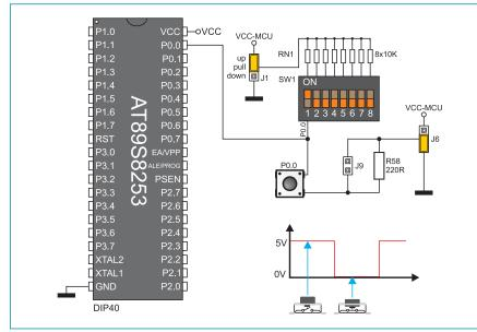
Figure 17-6: Jumper J1 in pull-up and jumper J6 in pull-down position
