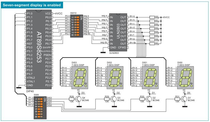
Figure 16-4: Seven-segment display connection schematic
