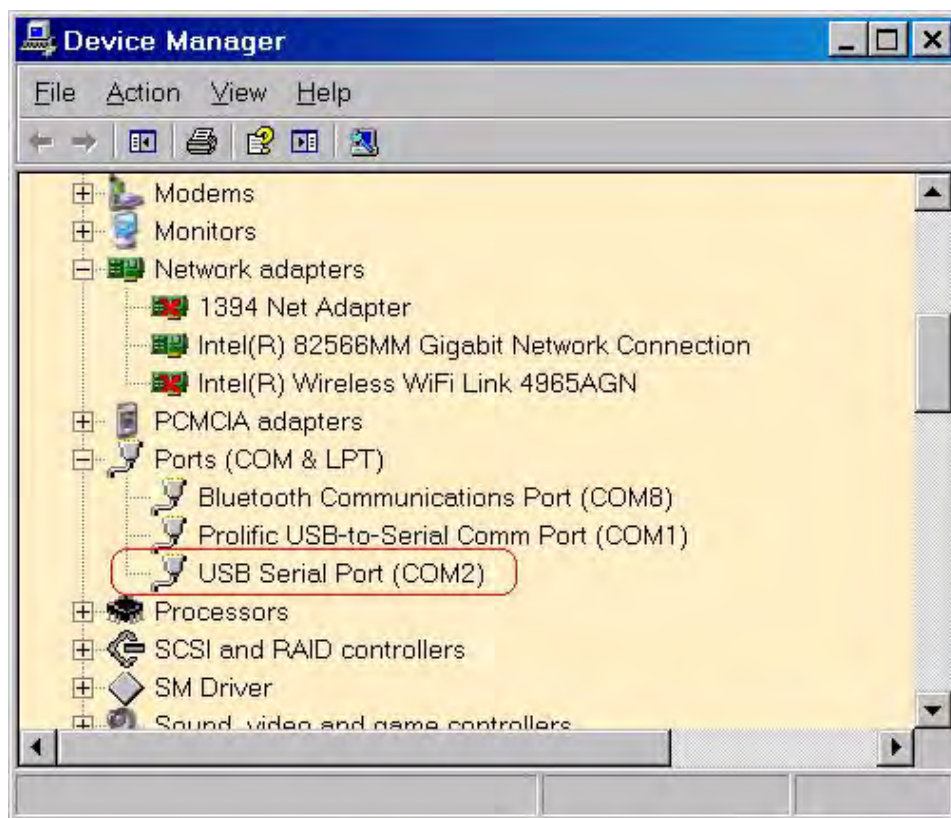
Figure 11. A Successful USB-to-UART Driver Installation
