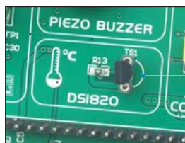
Figure 6-2: Temperature sensor DS1820 is connected
