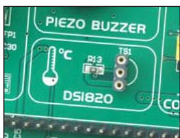
Figure 6-1: DS1820 connector (DS1820 is not connected)
