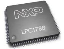
The NXP LPC1788 ARM Cortex-M3 based microcontroller runs the open source uEZ<sup>®</sup> + FreeRTOS software platform. The LPC1788 has 512KB of internal Flash memory, 96KB of internal SRAM, a 10/100 Ethernet Media Access Controller (MAC), a USB full speed device/host/OTG controller, four UARTs, two CAN channels and a collection of serial communications interfaces. The uEZ GUI board also includes 8MB of external SDRAM and 8MB of external NOR Flash.
