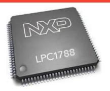
The NXP LPC1788 ARM Cortex-M3 based microcontroller runs the open source uEZ® + FreeRTOS software platform. The LPC1788 has 512KB of internal Flash memory, 96KB of internal SRAM, a 10/100 Ethernet Media Access Controller (MAC), a USB full speed device/host/OTG controller, four UARTs, two CAN channels and a collection of serial communications interfaces. The uEZ GUI board also includes 8MB of external SDRAM and 8MB of external NOR Flash.
