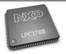
The NXP LPC1788 Cortex M-3 based microcontroller runs the open source uEZ® + FreeRTOS software platform. The LPC1788 has 512KB of internal Flash memory, 96KB of internal SRAM, a 10/100 Ethernet Media Access Controller (MAC), a USB full speed device/host/OTG controller, four UARTs, two CAN channels and a collection of serial communications interfaces. The uEZ GUI board also includes 8MB of external SDRAM and 8MB of external NOR Flash.
