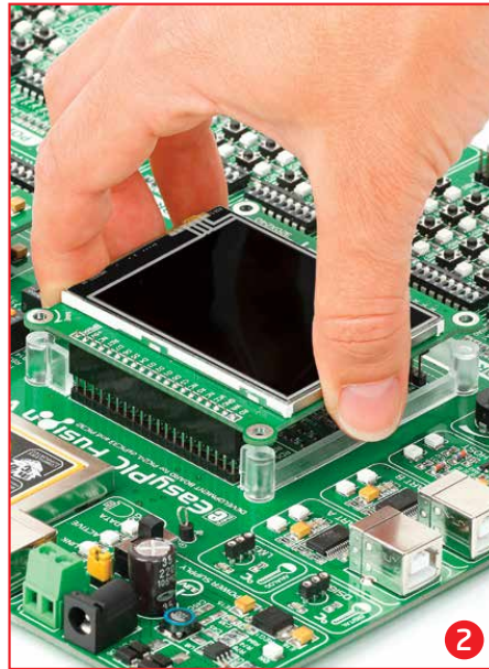
Figure 1-2: Place the EasyTFT board on the socket so that pins are aligned correctly.
