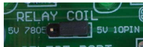
FIG1: Power selection jumpers
