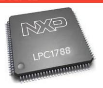
The NXP LPC1788 ARM Cortex-M3 based microcontroller runs the open source uEZ® + FreeRTOS software platform. The LPC1788 has 512KB of internal Flash memory, 96KB of internal SRAM, a 10/100 Ethernet Media Access Controller (MAC), a USB full speed device/host/OTG controller, four UARTs, two CAN channels and a collection of serial communications interfaces. The uEZ GUI board also includes 8MB of external SDRAM and 8MB of external NOR Flash.
