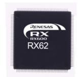
The **uEZGUI-RX62N-35OT** includes a 96MHz Renesas RX62N microcontroller running the open source uEZ® + FreeRTOS software platform. The RX62N has 512KB of internal Flash memory, 96KB of internal SRAM, a 10/100 Ethernet Media Access Controller (MAC), a USB full speed device/host/OTG controller, up to six UARTs, one CAN channels and a collection of serial communications interfaces.
