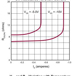
On-Resistance vs. Drain Current
