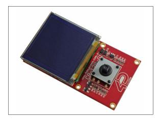
The **CB-160-G1** is a compact carrier board designed to provide a simple means of adding user input to the already capable uOLED-160-G1(SGC) (Serial Platform) and the uOLED-160-G1(GFX) (4DGL Platform) range of intelligent display modules. The tiny 5-position joystick, along with an on-board speaker, facilitates user input and output for these displays.
